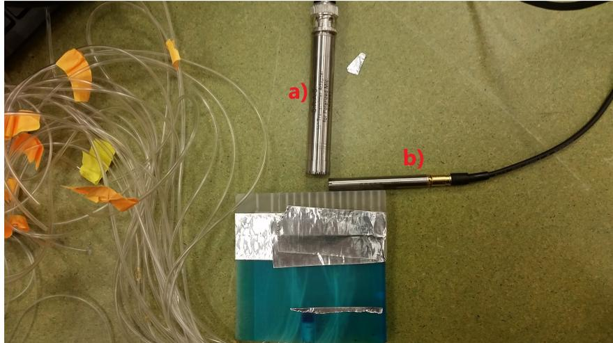
Figure 3.10: Close up, birds-eye view of the calibration setup. Note the perpendicular positioning of the a)reference speaker, b)reference microphone, and the model taps.
