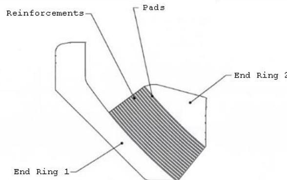
**Figure 1 Flexseal assembly example.**
