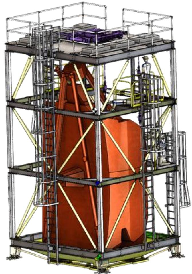
Contamination Tent designed to withstand acoustic loading and limit high frequency loading to sensitive instrument microshutters.
