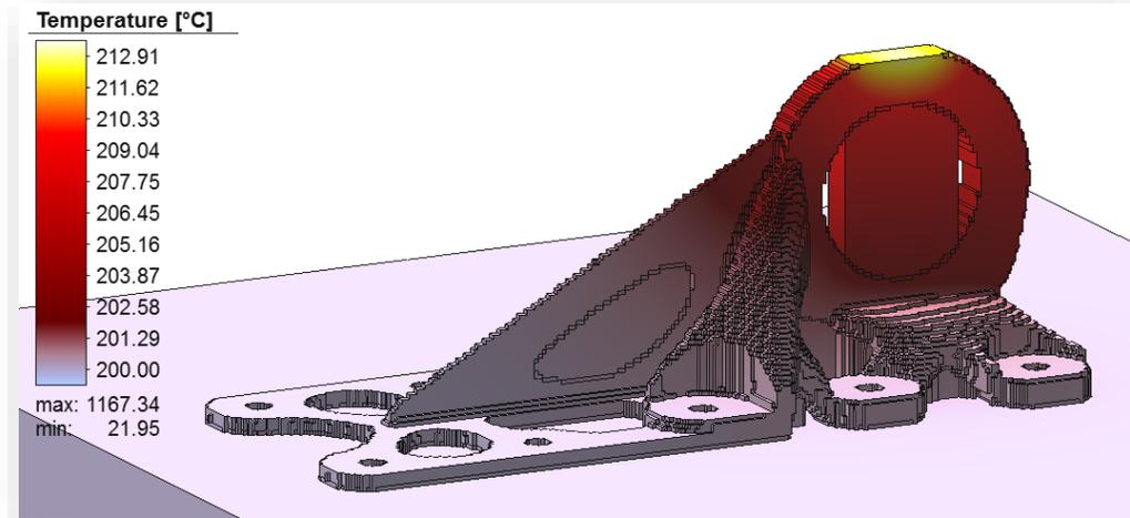
Secondary heat flux application – dissipation from top to bottom
