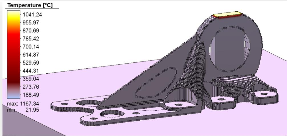
Primary heat flux application – melting
