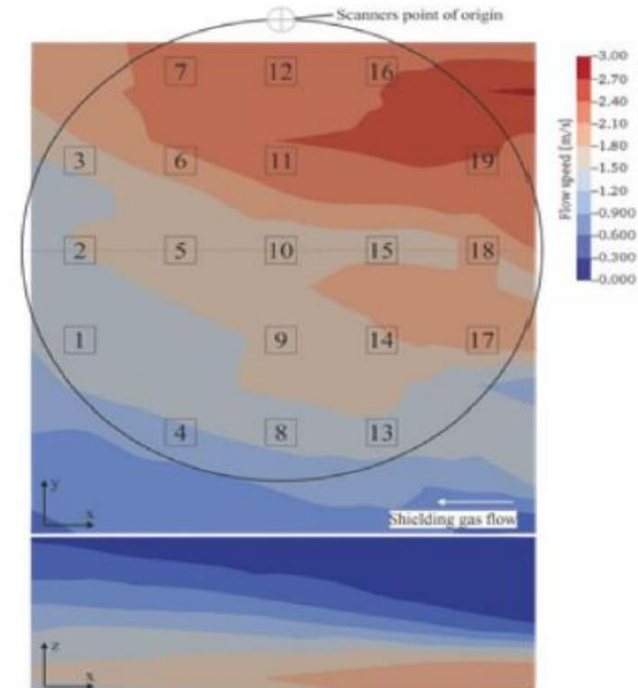
Measured shielding gas flow velocity distribution\*
