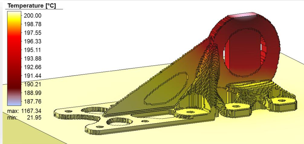
Cooling between layers (recoating time)
