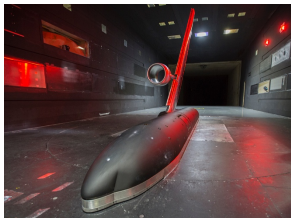
10-percent-scale High-Lift version of the NASA Common Research Model (CRM-HL) in Langley’s 14-by-22-Foot Subsonic Tunnel
