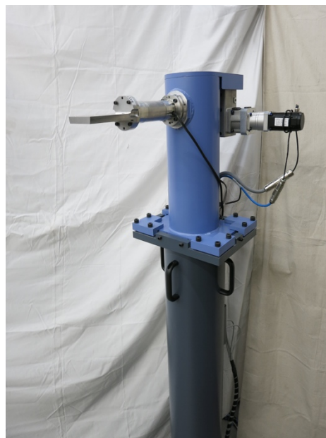
Sidewall model positioning system with the model block adapter installed.
