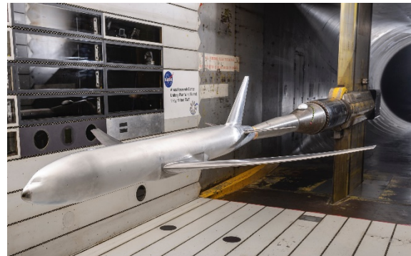
Ames Check Standard Model Installed in the 11-ft Transonic Wind Tunnel at NASA Ames
