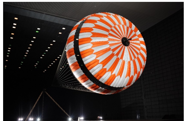
Mars 2020 canopy in flight in the NFAC 80- by 120-foot Wind Tunnel.
