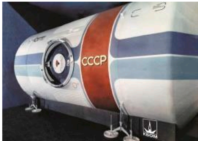
Fig. 15. A full-scale mockup of a Zvezda module and interior arrangements. (Credit: Barmin Design Bureau of General Engineering).
