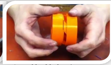
Assembly of fuel grain segments prototype - no build limits
