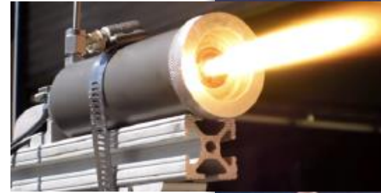
Thruster Installed In MSFC Test Cell C Vacuum Chamber
