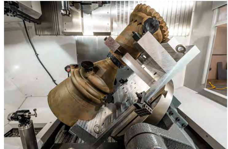
Photo: Launcher E-2 Combustion Chamber inside the Haas UMC-1000 CNC Machine.
