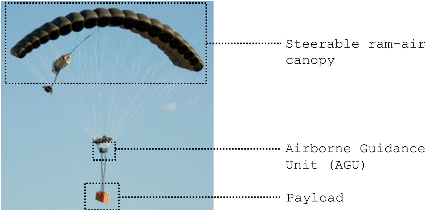
Figure 4: Autonomous parafoil with attached payload
