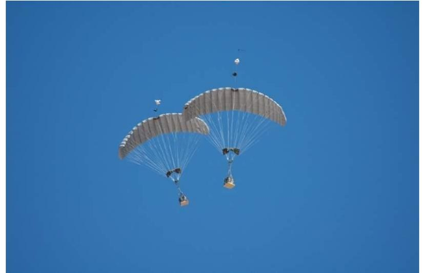
Figure 3: Guided airdrop with autonomous parafoils
