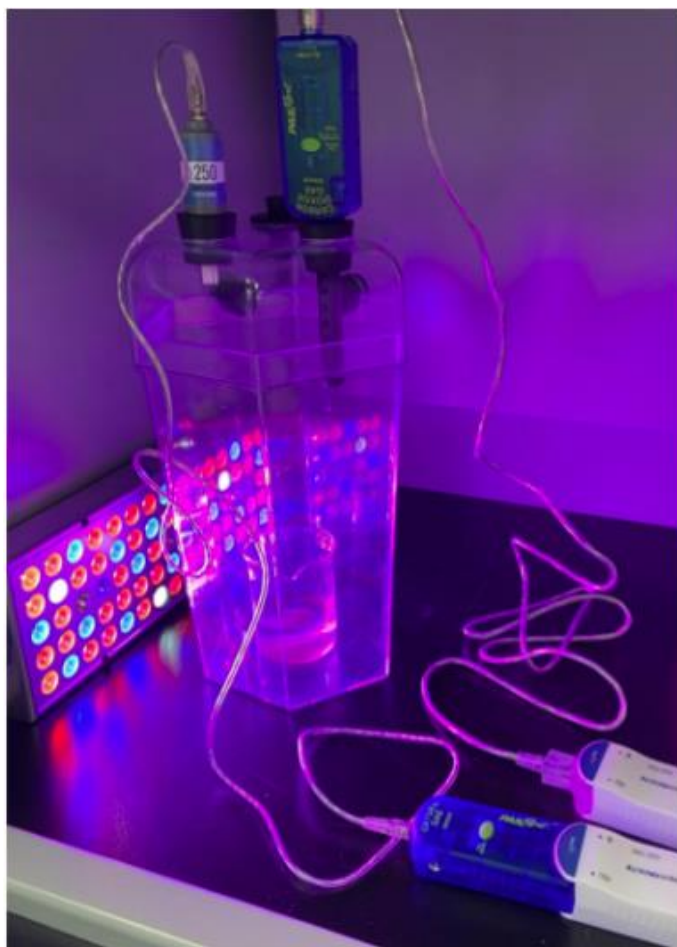
Alice Lentz's test apparatus for studying how algae affected the amount of airborne carbon dioxide and oxygen in a sealed environment.
