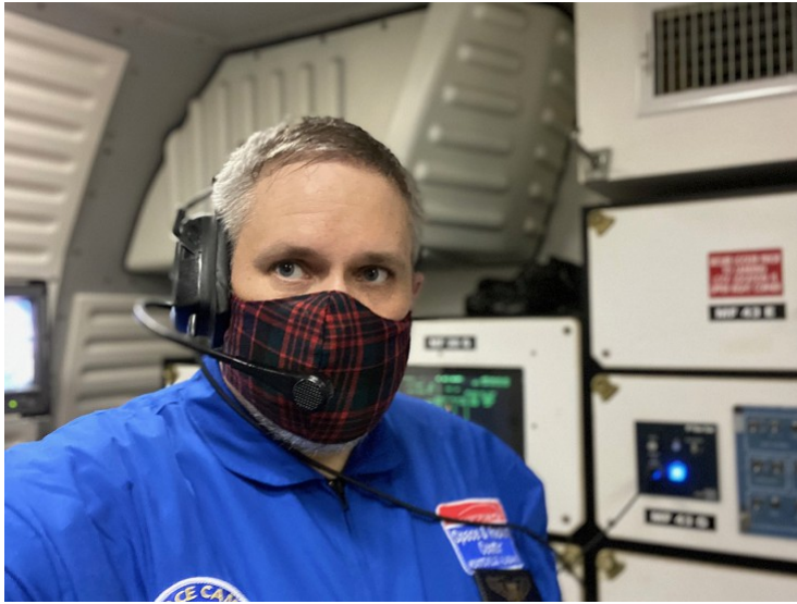
The shuttle trainer used for the simulated mission is a switch-for-switch replica of Columbia on STS-1. (Courtesy of David Hitt)
