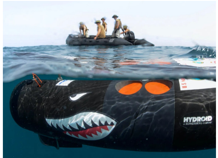
Members of the Naval Oceanography Mine Warfare Center at Stennis Space Center, Mississippi, standing by as an unmanned underwater vehicle leaves the surface to search for mines. Photo: AFP/Gary M Keen/US Navy
