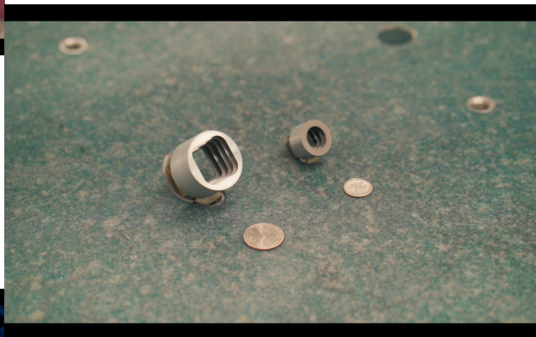
(Right) Cold Shield close with dimes: is a component used for the SM-3 Targeting system
