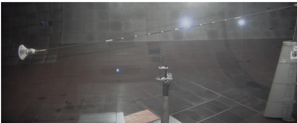
The ASDRS/ORS system under test in the NFAC 40- by 80-foot Wind Tunnel
