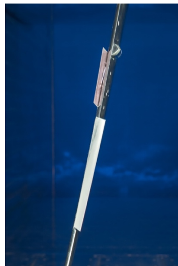
Remote control actuated aileron and outboard spoiler using shape memory alloy technology
