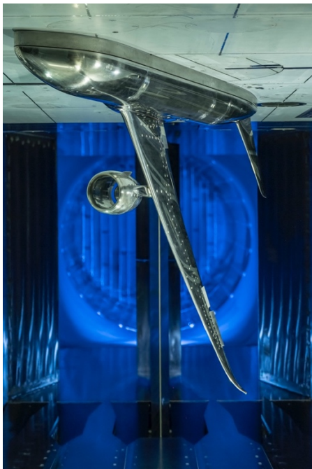
SMA-based RCA spoilers and aileron on a half-span Boeing transport model in ETW
