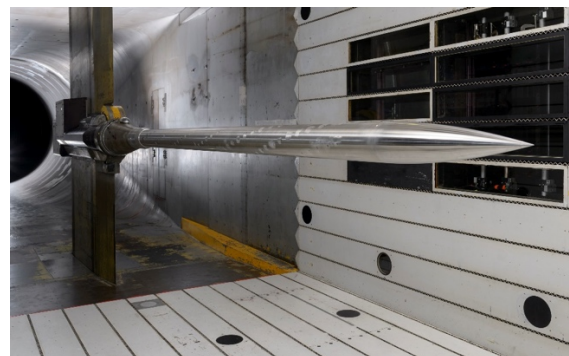
9-foot short static pipe used for calibration check standard testing
