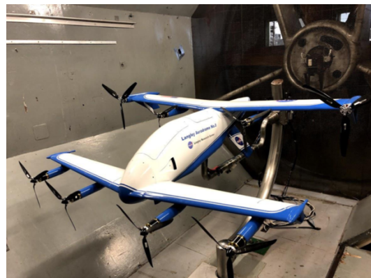
The LA-8 model in the NASA Langley 12-Foot Low Speed Tunnel
