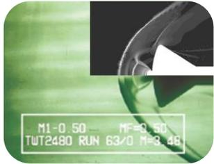
Re-entry capsule with counter-flowing jet, Mach 3.5, Turbulent, Air as ideal-gas (Daso case)
